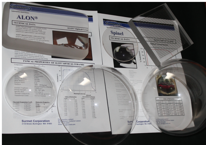
FIGURE 1. Examples of ALON and spinel components produced by Surmet are shown, including a component with a metal grid incorporated into it (upper right). (Courtesy of Surmet)
