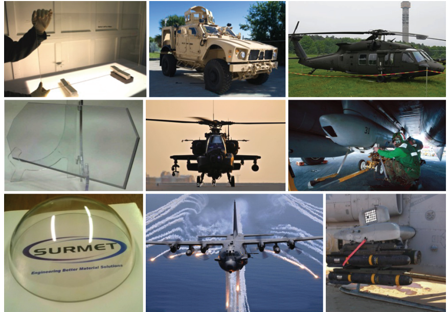
FIGURE 3. Examples of ALON transparent ceramic components and their applications (top row: transparent armor; middle: sensor and reconnaissance windows; bottom: mid-IR optics for missiles and countermeasures). (Courtesies: Left column: Surmet. Middle: Joe Bullinger, U.S. Navy (top); U.S. Air Force photo/ Matt Hecht (middle); Julianne Showalter, U.S. Air Force (bottom); and Right: Bengt Oberger (top); Brian Fleske, U.S. Navy (middle); Looper5920 (bottom). Middle and right columns via Wikimedia Commons.)
