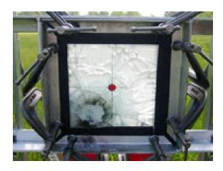
A chemical compound of oxygen and aluminum, called alumina, makes a strong shield. (Air Force Research Labs)
