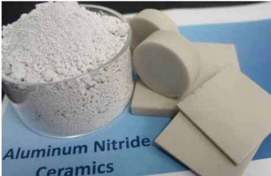
Figure 1. Aluminum nitride powder and sintered components manufactured by Surmet (Burlington, Mass.).
