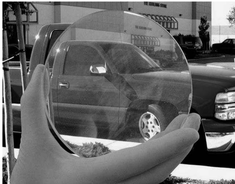
Figure 3: Spinel lens produced using production process
