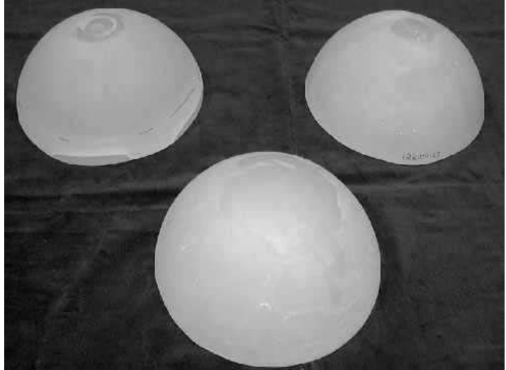
Figure 5: Several 7" spinel dome blanks for JCM
