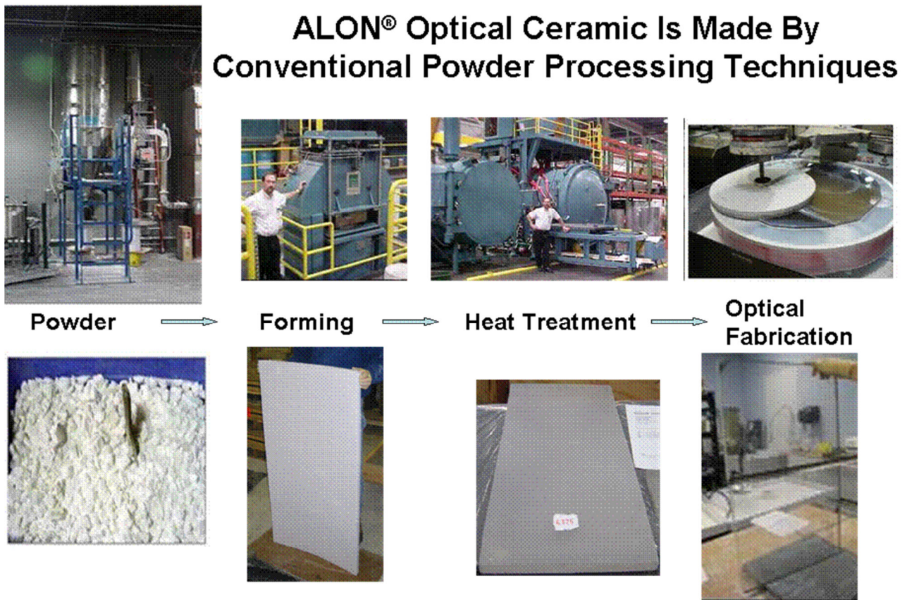
Figure 2: Schematic of process for producing ALON by powder processing
