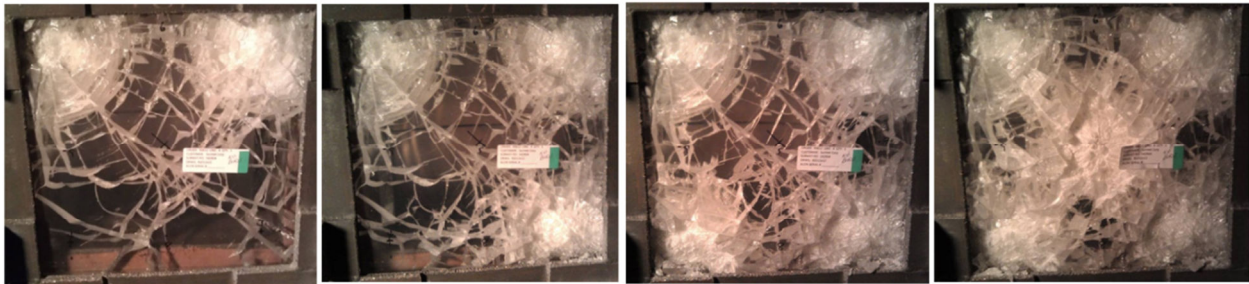
Figure 12: Shot sequence on 12x12-in ALON Armor Laminate, after 2, 3 4 and 5 shots. 4 additional shots were also successfully stopped by this laminate
