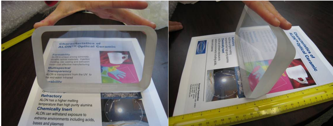
Figure 10. Photograph of 1.3-in thick ALON ® window from the front and side
