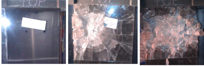
Figure 11: Photographs of 6x6-ALON ® Armor laminate prior to shooting (left) after first shot (center) and after 2 nd shot (right)
