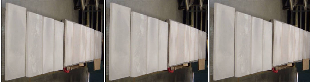
Figure 3: Three photographs of 11 large ALON ® blanks produced for Recce applications representing the nearly tripling of Surmet production capacity for these windows
